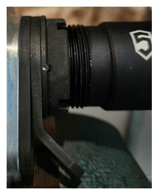
8) **Reinstall Buffer and Buffer Spring**: install the buffer and spring into the Buffer Tube, making sure that the face of the buffer has past and is contacting the Buffer Retainer.
